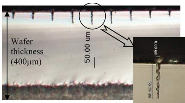
FIG. 4. Edge-view cross-sectional picture of scribe depths corresponding to various focal planes.
