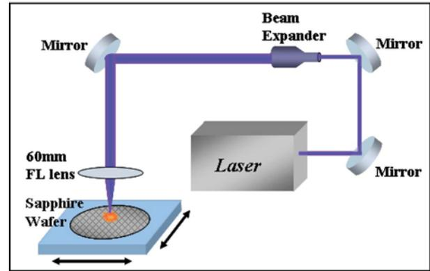
FIG. 2. Experimental optical setup for LED sapphire wafer scribing.
