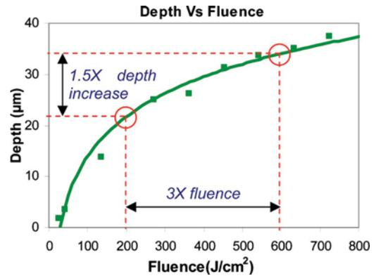
FIG. 10. Plot illustrating the inefficiency expected with excessive fluence levels.
