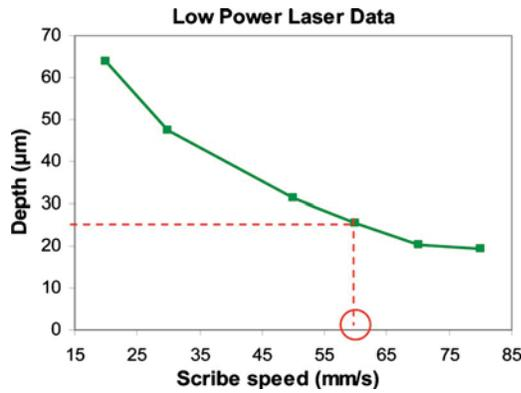
FIG. 8. Plot of scribe depth vs scribe speeds for the Tristar 355-3 laser operated at 150 kHz.
