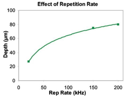
FIG. 7. Plot of scribe depth vs repetition rates showing advantage of high repetition rate.
