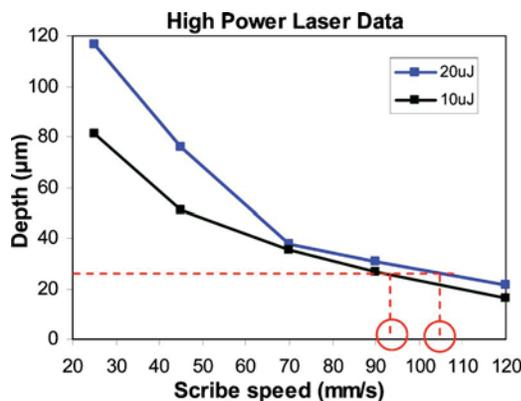
FIG. 9. Plot of scribe depth vs scribe speeds for Pulseo laser operated at 200 kHz.
