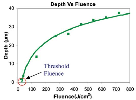
FIG. 5. Plot of scribe depth as a function of laser fluence illustrating the threshold fluence.
