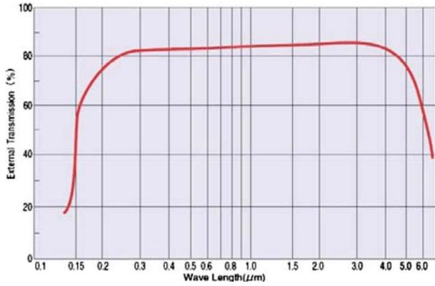
FIG. 1. Transmission versus wavelength curve for 1mm thick sapphire wafer.
