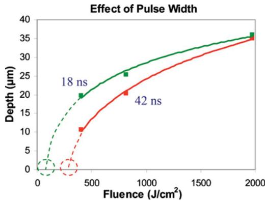
FIG. 6. Plot of scribe depth vs fluence, showing advantage of short pulse widths.
