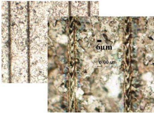
FIG. 3. Top-view microscope picture of example scribes on sapphire wafer.
