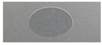
Figure 1: 10 mm diameter hole cut out in 200  $\mu m$  thick Corning Willow glass
