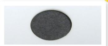
Figure 3: Digital camera photo of 5 mm diameter hole machined in 200  $\mu$ m thick alumina ceramic plate shows very good edge quality and no discoloration of the material.
