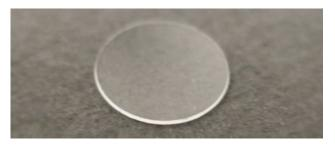
Figure 2: Macro camera photo of 5 mm disk cut from a 150 µm thick sapphire wafer
