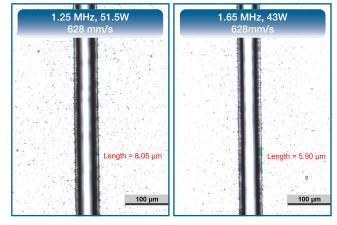
Figure 1 PET film cut with lower (left) and higher (right) laser pulse frequencies.
