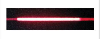
Figure 5: Photograph of an optical fiber diffusor with a length of 55.5 mm fabricated with the Spirit femtosecond laser. Light is decoupled out of the optical fiber at the modified areas and results in a uniformly diffused illumination.
