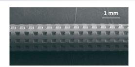
Figure 3: SEM (scanning electron micrograph) image showing a detailed view of a modified area. Shown are machined defects with a footprint of 250 x 250  $\mu$ m and a depth of 65  $\mu$ m. The bottom surface is in the fiber core so that light is decoupled because the total internal reflection is prevented.
