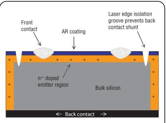
Without edge isolation groove, current shunt occurs between front and back contact through the ion diffusion layer
