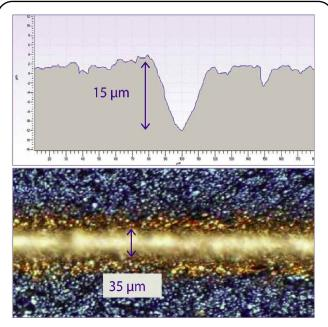
Depth profile (top) and microscope photo of edge isolation groove machined with Pulseo 355-20 laser system.
