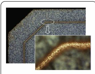
Low- and high-magnification optical microscope images of 532-nm laser edge isolation scribe
