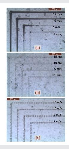
Figure 2. Microscope images showing one corner of a  $1 \times 1$  mm square processed with a UV ultrafast laser with (a) free running, (b) skywriting and (c) PSO techniques.
