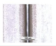
Figure 3. Full cut in 45–50  $\mu$ m thick bare LCP sheet material with a single pass at 1.0 m/s scan speed.
