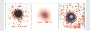
Figure 1. Blind via in Cu/MPI/Cu laminate with microscope focus on the top copper (left) and bottom copper (middle); through-hole via imaged at the top copper surface (right).
