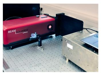
Fig. 3: The beam profile of the femtosecond lasers is checked with the Ophir BeamSquared analysis system.
