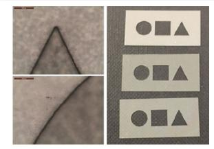
Figure 3. Microscope images of Polyethylene Terephthalate (PET) plastic ribbon cut using a femtosecond Spirit 1030-100-SHG laser at 515 nm. The average power of 50 W at 515 nm results in cutting speeds over 0.4 m/s for 75 µm thick PET with superior quality (HAZ <10 μm).
