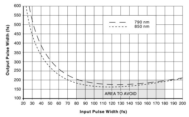
Figure 3-3: Output pulse width from the AOM as a function of input pulse width.
