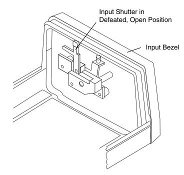
Figure 2-3: The Model 3980 Interlock Shutter
