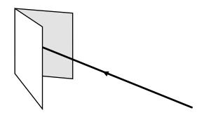
Figure 2-2: Folded Metal Beam Target
