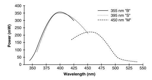
Figure 3-4: Typical frequency-doubled, Tsunami ps tuning curves using 10 W TEM<sub>00</sub> pump power from a Millennia Xs.
