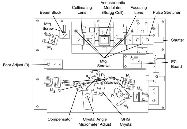
Figure 4-2: Model 3980 Optical Elements
