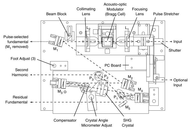
Figure 3-1: Model 3980 Schematic and Optical Beam Path
