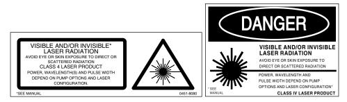
Figure 2-1: These CE and CDRH standard safety warning labels would be appropriate for use as entry warning signs (EN 60825-1, ANSI 4.3.10.1).
