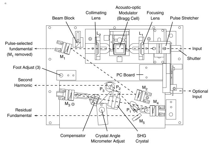
Figure 1-2: Model 3980 Schematic and Optical Beam Path
