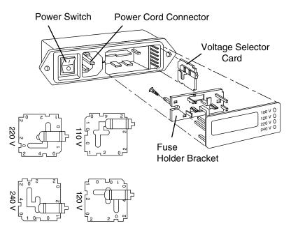
The four orientations of the voltage selector card.
