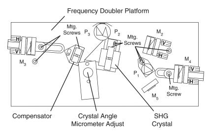
**Figure 4-5: Frequency Doubler Components and Controls**
