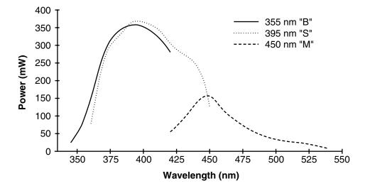
Figure 3-5: Typical frequency-doubled, Tsunami fs tuning curves using 10 W  $\text{TEM}_{00}$  pump power from a Millennia Xs.
