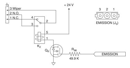
Figure 4-8: Model J80 Emission Connector Circuit
