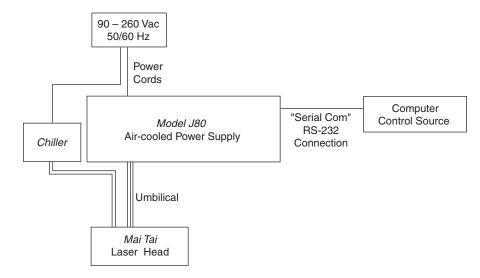
Figure 5-6: The *Model J80* Interconnect Drawing
