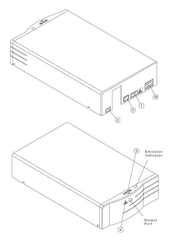
Figure 2-8: CE/CDRH Radiation Control Drawing, Scientific Version (labels shown on page 2-10)
