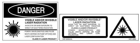
Figure 2-1: These CDRH and CE standard safety warning labels would be appropriate for use as entry warning signs (ANSI 4.3.10.1, EN 60825-1).
