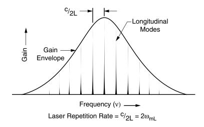
Figure A-3: Amplitude and frequency of longitudinal modes in a modelocked laser.
