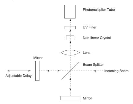
Figure B-1: Interferometric (Collinear) Autocorrelation
