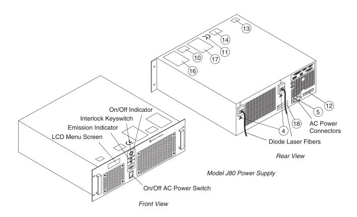
Figure 2-9: CE/CDRH Radiation Control Drawing, *Model J80* Power Supply (labels shown on page 2-10)
