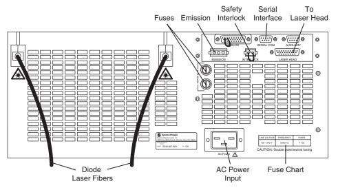
Figure 4-5: The *Model J80* Power Supply Rear Panel
