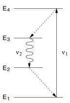
Figure 3-2: A Typical Four-level Transition Scheme
