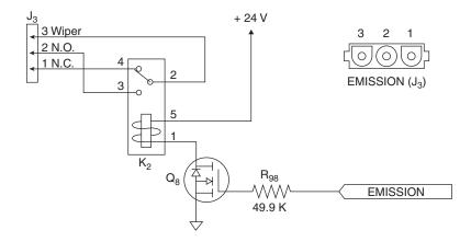
Figure 2-4: The EMISSION Connector Schematic
