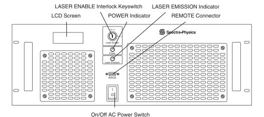
Figure 4-4: The *Model J80* Power Supply Front Panel
