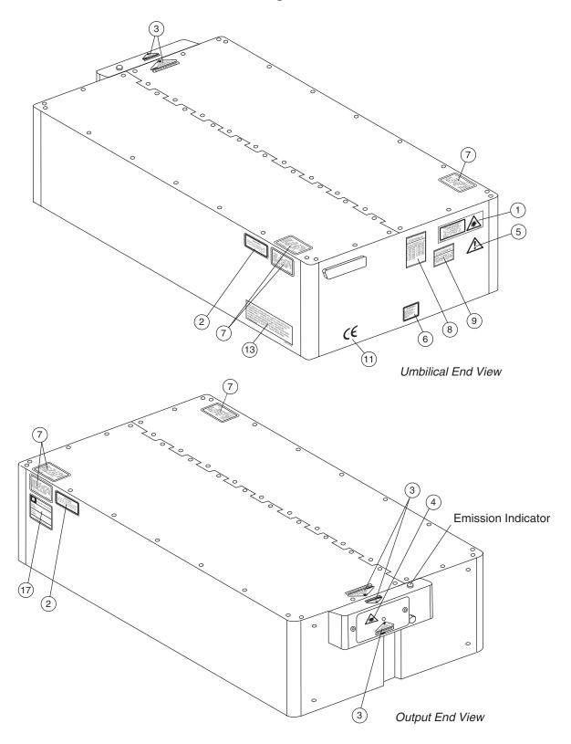
Figure 2-7: CE/CDRH Radiation Control Drawing, OEM Version (labels shown on page 2-10)
