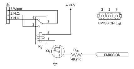
Figure 5-9: The EMISSION Connector Schematic
