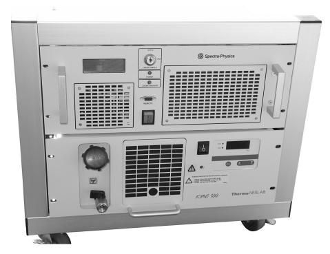
Figure 5-5: The Power Supply and Chiller in the Rack
