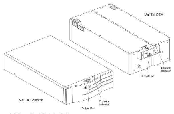
Figure 2-3: Laser Head Emission Indicator
