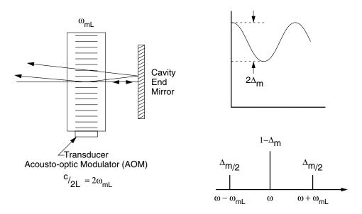
Figure A-2: Active modelocking using an AOM. Modulation sidebands are produced when a wave passes through an amplitude modulator.
