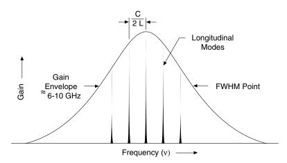
Figure 3-3: Frequency Distribution of Longitudinal Modes for a Single Line
