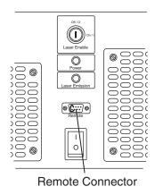
Figure 5-7: The REMOTE Connector on the Power Supply Front Panel
