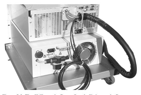
Figure 5-3: The Chiller and a Power Supply Sitting on the Base
