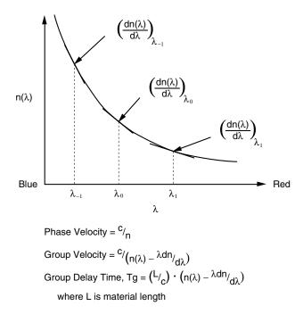
Figure A-5: Typical wavelength dependence of the refractive index of a material.
