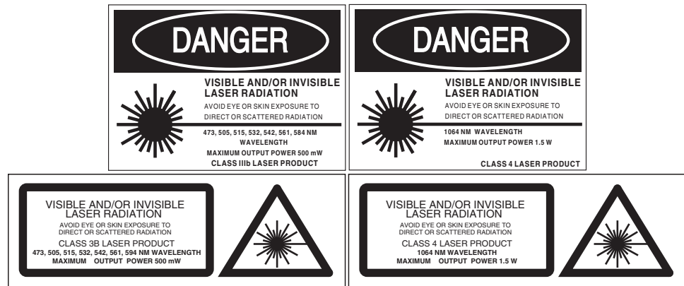
Figure 2-1: These standard safety warning labels are appropriate for use as entry warning signs (EN 60825-1: 2007, ANSI Z136.1, Section 4.7).
