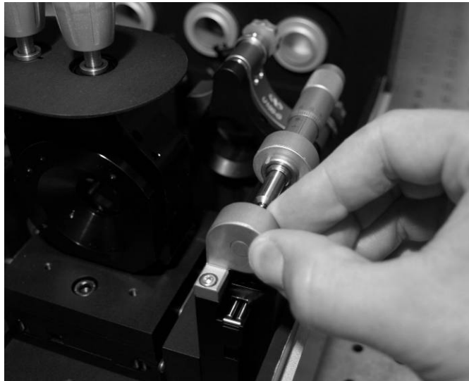
Figure V.3: Sliding the alignment cavity output coupler to observe a flash.
