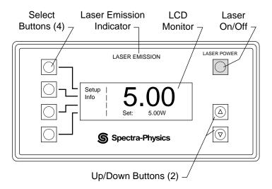
Figure 6-1: The Millennia IR Controller Showing the Default Main Menu.
