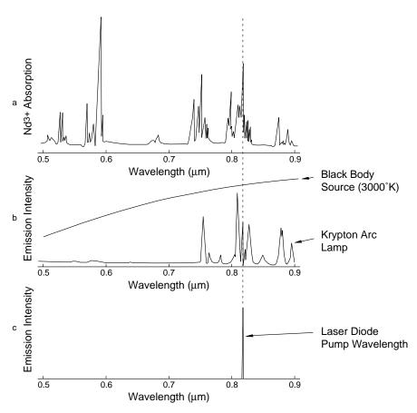
Figure 3-5: Nd<sup>3+</sup> absorption spectra compared to emission spectra of a Black Body Source (a), Krypton Arc Lamp (b) and a Laser Pump Diode (c).
