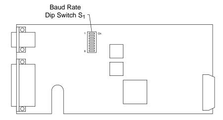
Figure 6-3: Laser head pc board showing the location of baud rate dip switch  $S_1$ .
