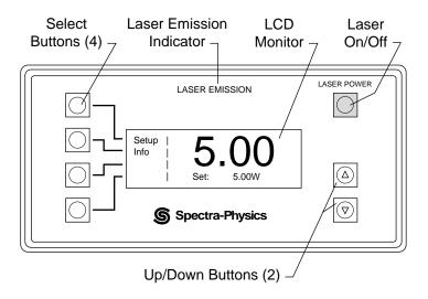
Figure 4-3: The Millennia IR Control Module
