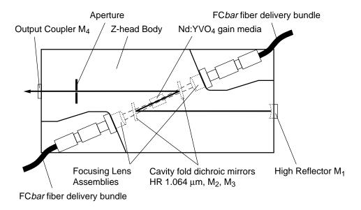
Figure 3-10: The Z-Head (top view)
