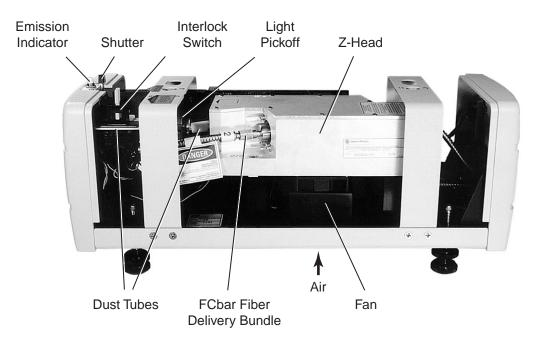
Figure 4-1: The Millennia IR Laser Head
