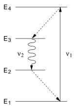
Figure 3-2: A Typical Four-level Transition Scheme
