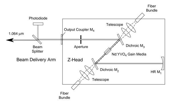
Figure 3-9: Schematic of the Millennia IR Laser Head
