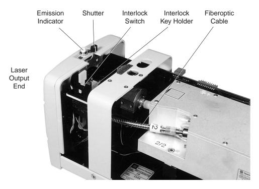
Figure 2-4: Laser Head Emission Indicator, Shutter and Safety Interlock
