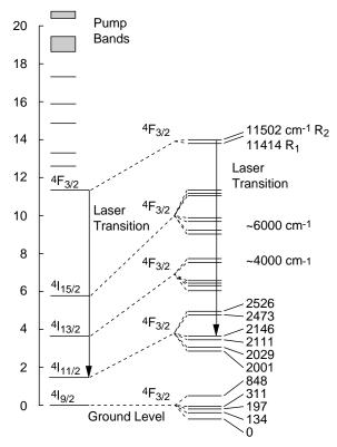
Figure 3-4: Energy Level Scheme for the Nd<sup>3+</sup> Ion.
